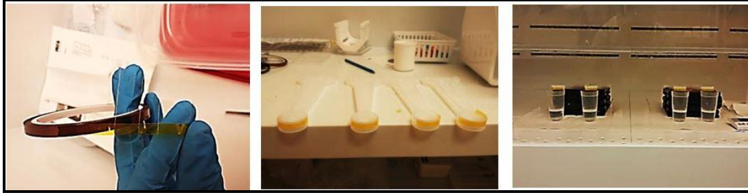
Figure 9 Various steps involved in fabrication of nanoendoscope. First, cleaved optical fibers are loaded onto the capton tape. Next tape with optical fibers is affixed onto a Teflon holder. Finally, the Teflon holder placed in solution of HF. The process is timed after insertion of holder with fibers into HF.
